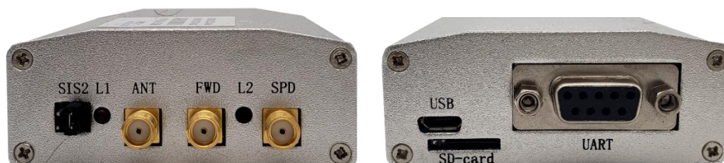
Figure 3-1 Interfaces & Indicators on UM220-INS NL EVK
